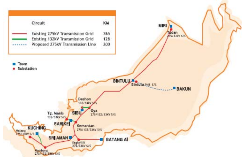
Figure 1: Main Grid System in Sarawak
